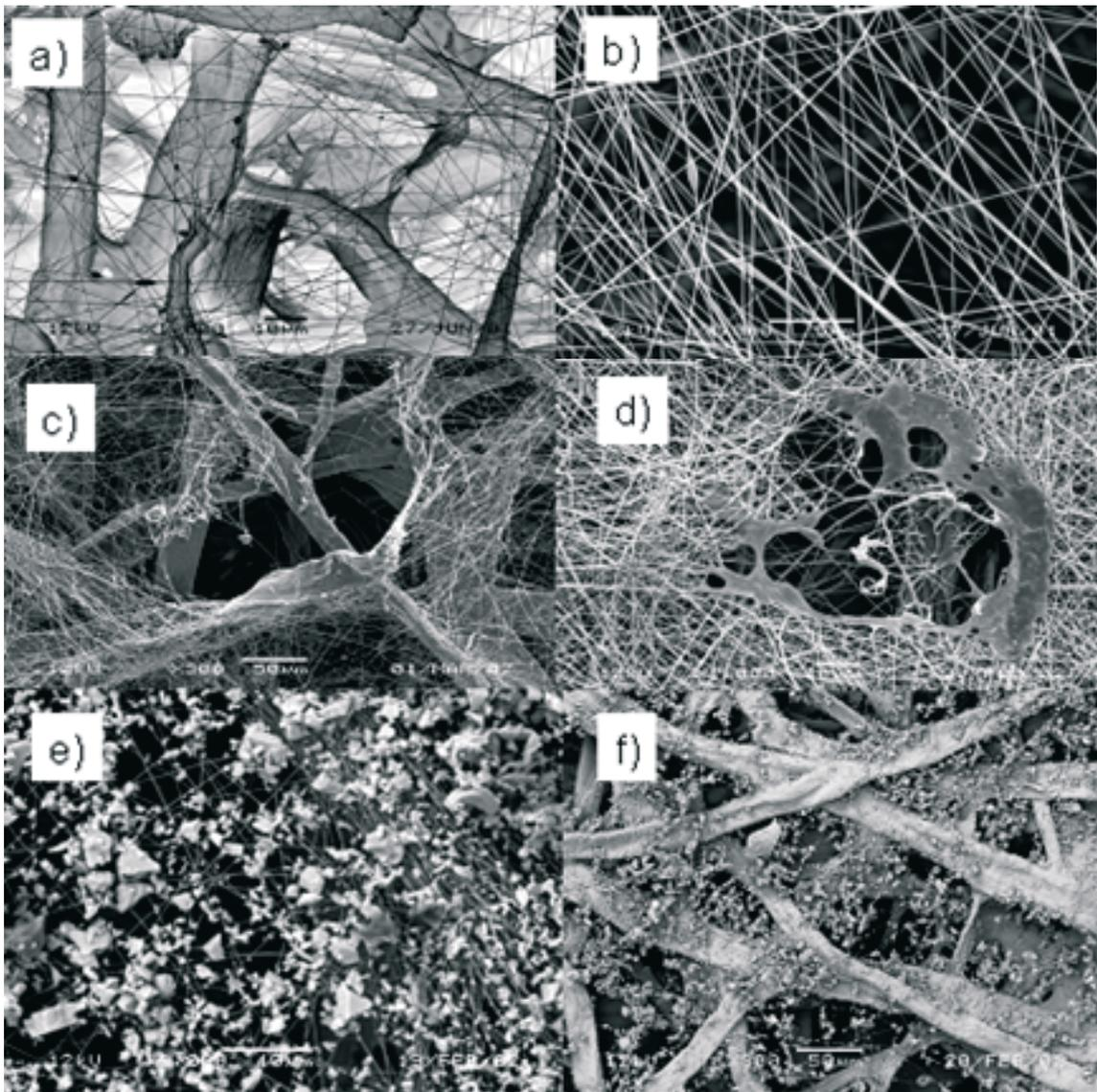
Fig. 4. Uniform (a and b) and non-uniform (c and d) nanofiber and dust cake distribution (e and f)
