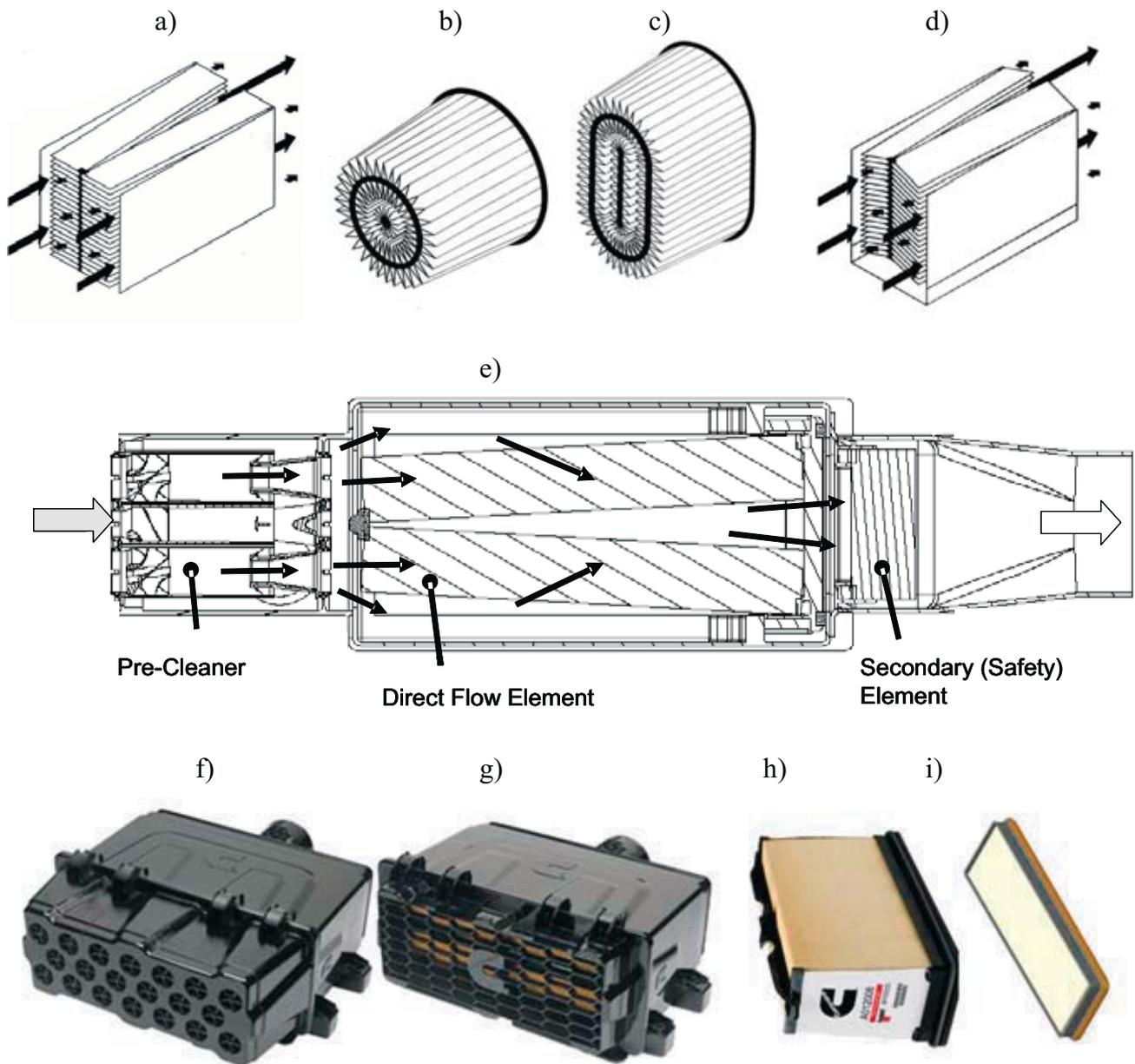
Fig. 1. Schematic and full view of Direct Flow filters; a) flow pattern through a rectangular filter with 2- filter elements, b) multi cylindrical filter, c) elliptical multi element filter ,d) filter element with skewed pleats, e) schematic view of filter assembly, f) Direct Flow filter with through flow cyclonic precleaner, g) Direct Flow filter with inlet grate, h)filter element, i) secondary (safety) filter
