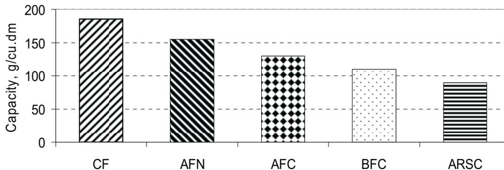
Fig. 2. Dust capacity of fluted and Direct Flow Filters, CF - Direct Flow filter, HD cellulose filter media, AFN company A, commercial fluted filter, nanofiber filter media, company A, commercial fluted filter, cellulose filter media, BFC - company B, commercial fluted filter, Cellulose filter media, ARSC - company A, commercial radial seal cylindrical filter
