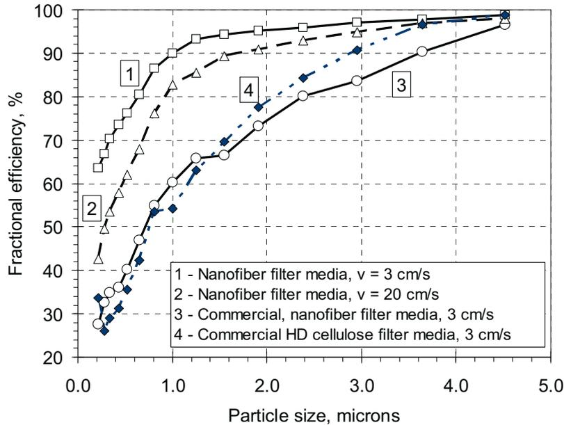
Fig. 3. Fractional efficiency of pleatable filter media
